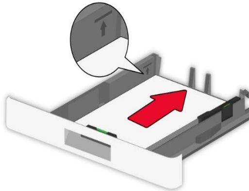
4. Adjust the guide to match the size of the loaded paper.
