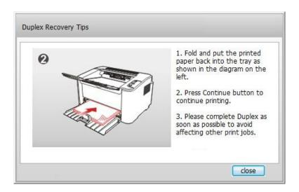
f) After turning over the paper according to the prompt, press Continue button of the printer to go on printing the other side.
